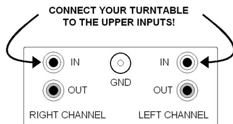
Now connect a good pair of unbalanced interconnects from the outputs to a pair of line level inputs on your amplifier.
